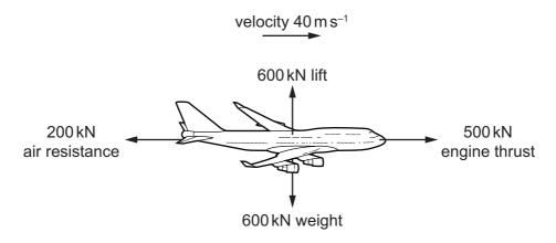
At which rate is its kinetic energy increasing?
