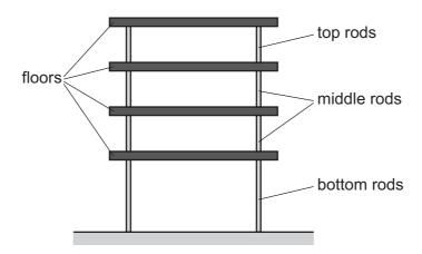
The spacing of the bottom floor from the ground is twice that of the spacing between the floors. Between each floor are equal numbers of vertical steel supporting rods of negligible mass compared with the floors. The rods are of different diameters so that the stress in each rod is the same.
