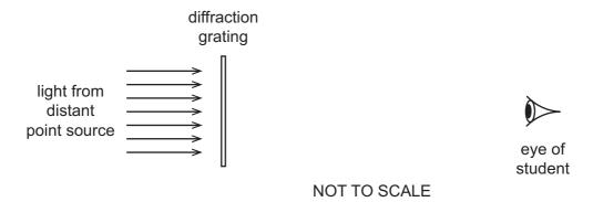
The plane of the diffraction grating is at right angles to the incident light. A student looks at the grating from a position near to the grating.
