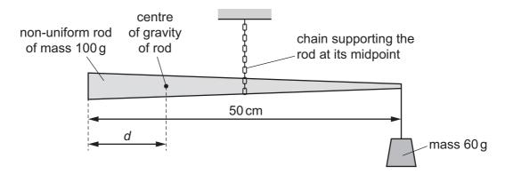
The centre of gravity of the rod is a distance *d* from its left-hand end.
