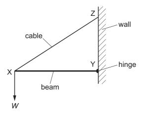
The beam supports a weight W at point X. The forces in the cable and the beam are  $F_C$  and  $F_B$  respectively.
