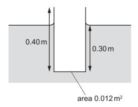
The cross-sectional area of the pipe is  $0.012\,\text{m}^2$ . The weight of the pipe is  $32\,\text{N}$ .
