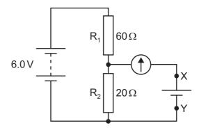
The circuit is to be used to test whether the electromotive force (e.m.f.) of a particular cell is 1.5 V. The cell is connected between terminals X and Y in parallel with  $R_2$  and in series with a galvanometer.
