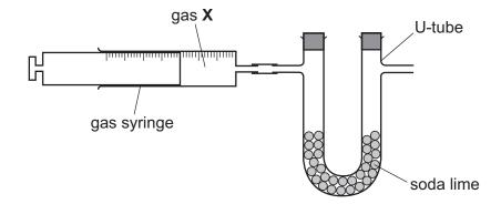
A 100.0 cm<sup>3</sup> sample of pure gas **X** is placed in a gas syringe. The gas syringe is attached to a U-tube containing small lumps of solid soda lime, a mixture of sodium hydroxide and calcium hydroxide. All of gas **X** is slowly passed into the U-tube and the mass of gas **X** absorbed determined.
