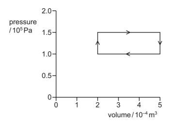
During the change when work is done on the gas by its surroundings, how much work is done on the gas?
