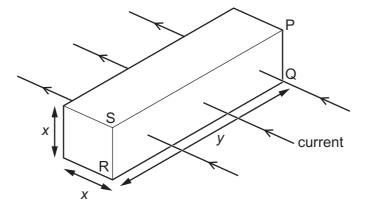
The number density of charge carriers is n. Each charge carrier has charge e. The average drift speed of the charge carriers is v.
