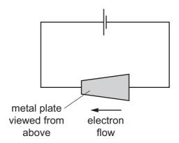
Electrons move clockwise around the circuit.
