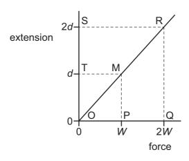
Initially a force W gives an extension d. The force is then increased to 2W. This increases the extension to 2d.
