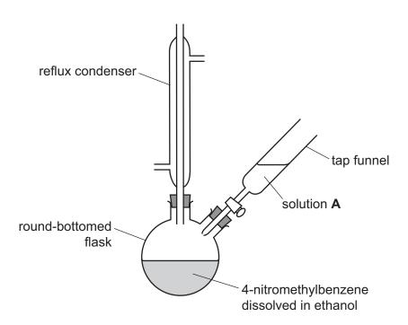
(a) (i) Show, using a labelled arrow, where the cooling water enters the reflux condenser. [1]
