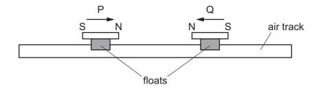
The two magnets slide towards each other along the air track and interact, without making contact.
