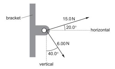
What are the magnitudes of the horizontal and vertical components of the resultant of the two forces?
