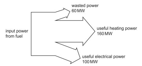
What is the efficiency of the CHP station for producing useful power?
