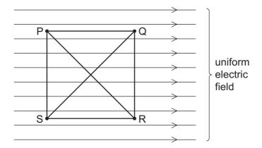
The charge moves along different straight paths between points P, Q, R and S.
