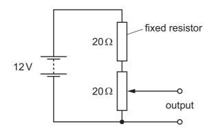
The fixed resistor and the potentiometer each have resistance  $20 \Omega$ . The circuit is designed to provide a variable output voltage.
