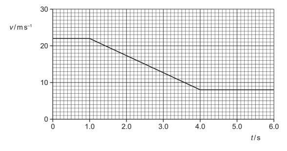
The brakes of the car are applied from t = 1.0 s to t = 4.0 s.
