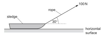
How much work does the boy do on the sledge when he pulls it a distance of 5.0 m along the surface?
