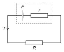
The resistance R and the e.m.f. E remain fixed. The internal resistance r of the cell changes over time.
