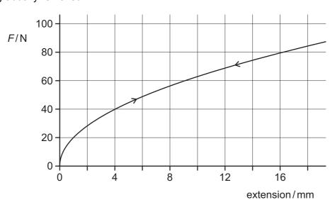
What is the best estimate of the strain energy in the rubber when a load of 80 N is applied?
