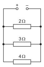
The power dissipated in each of the resistors of resistance  $2\Omega$ ,  $3\Omega$  and  $4\Omega$  is  $P_2$ ,  $P_3$  and  $P_4$  respectively.
