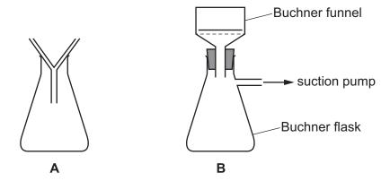
method A: gravity filtration using a filter funnel, filter paper and a conical flask
